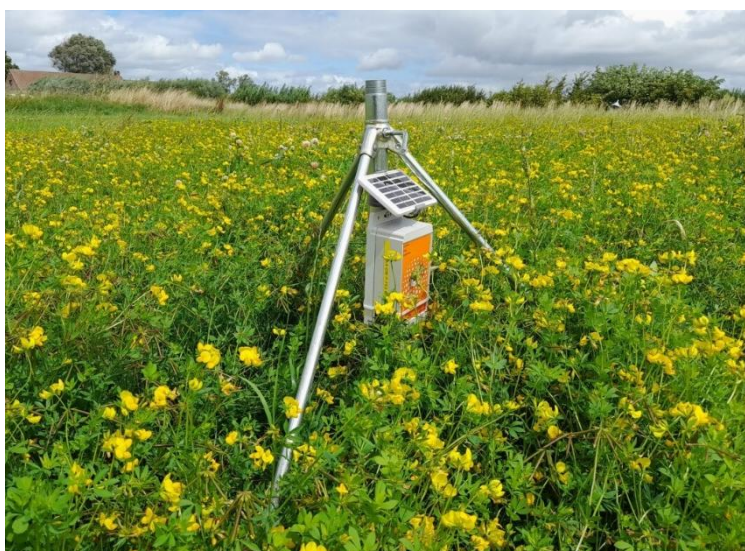
Figure 8: Test setup of the Polly sensor in a plot of clover.
