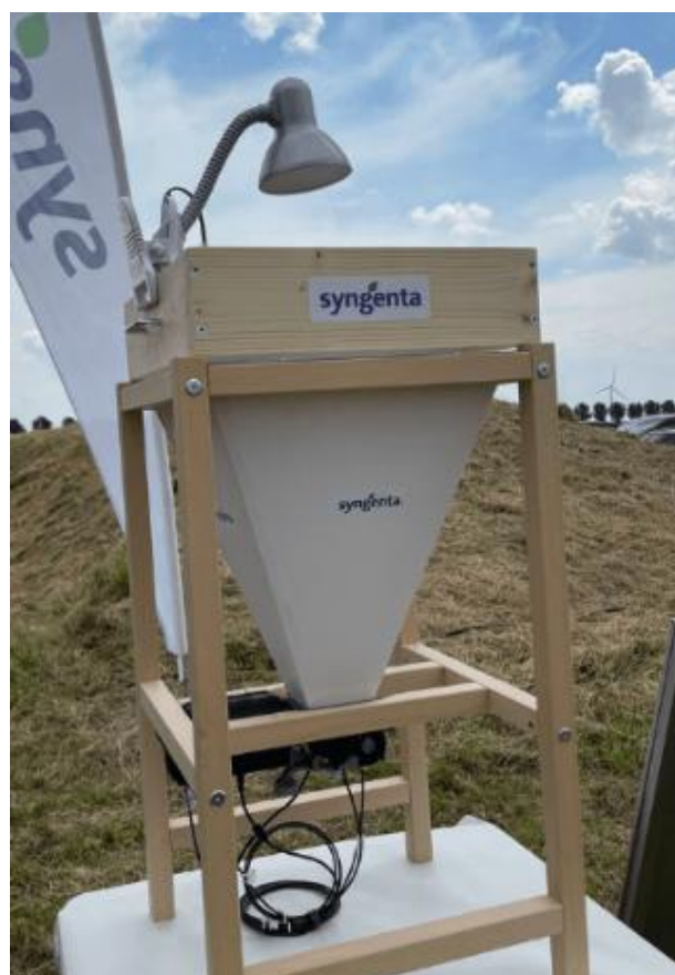
Figure 9: The Edapholog sensor.
