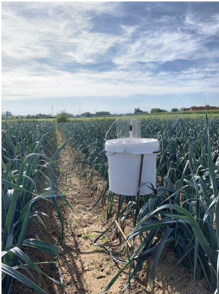
Figure 5: Setup of an LED bucket. The lamp automatically turns on when it gets dark.
