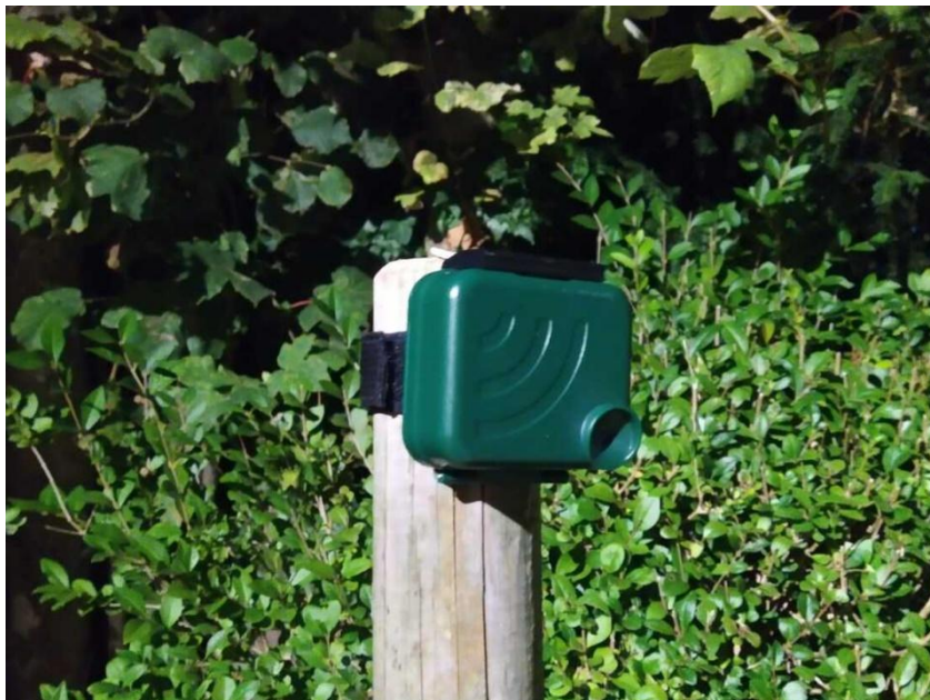
Figure 6: Audiomoth devices are mounted on a pole.
