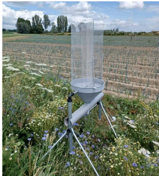
Figure 1: Window trap in operation (version 2023).
