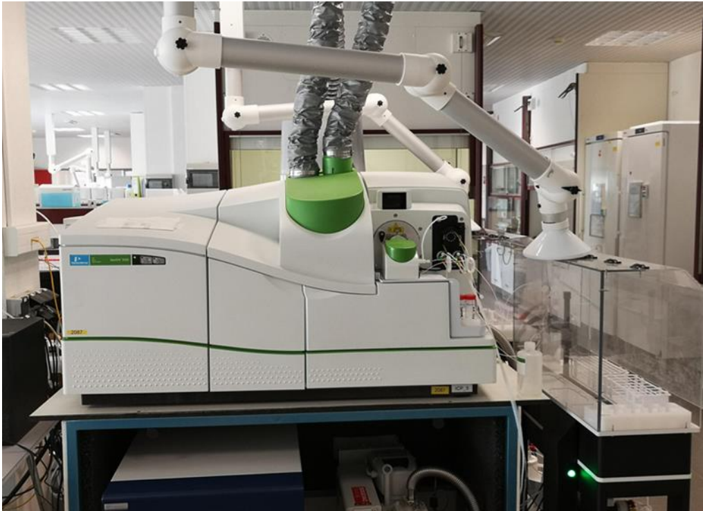
Figure 3: ICP-MS used to analyse the Rb-content in the individual insects.
